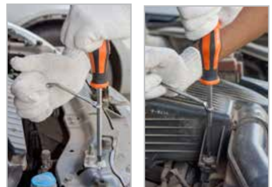
Hex shaft can be tightened using a spanner for high torque applications
